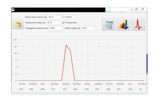
In addition to PD detection, the device can be used for on-line PD cable mapping to locate significant cable PD within 1% of the circuit's overall length.
