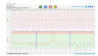
To increase your ability in assessing a machine's rotor/ mechanical performance, the HVPD Kronos® Spot Tester has an add-on Motor Current Signature Analysis (MCSA) feature – non-intrusive, on-line test technique, used to assess the rotor condition of motors by analysing the frequency content of the current.
